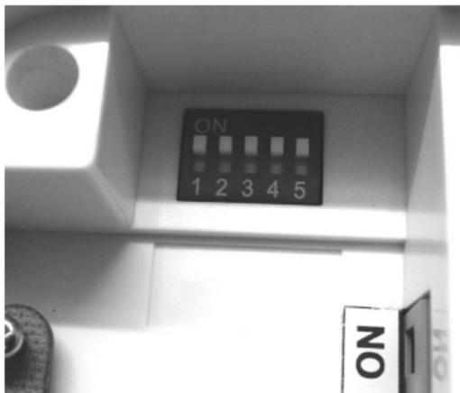
To adjust the RF address code of the Control Centre, remove one or more of the jumper caps located on the back of the unit (labelled 1,2,3,4 and 5, and shown in the picture below) so that the jumper settings match the settings made on the receiver:
