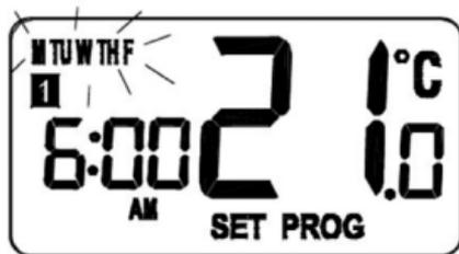
Press the UP or DOWN key to select the programme set for either Weekday or Weekend to be reviewed or adjusted. Pressing the SET key at any time when in programming mode will return the RT500RF into Normal mode.
