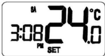
When operating in Temporary Override mode, the LCD display will show the temporary set point temperature:
