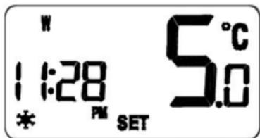
When operating in Frost Protection mode, the LCD display will show a reading of 5 °C and also display the Frost Protection indicator:
