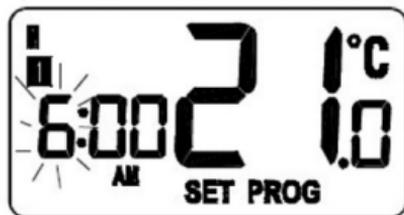
Press the UP or DOWN key to adjust the hour setting to the desired value, and confirm your selection by pressing the SELECT key.
