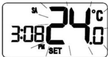
Pressing the UP or DOWN key will increase or decrease the set point temperature in 0.5 °C steps - the set point temperature can be adjusted within a set range of 10 °C to 35 °C.
