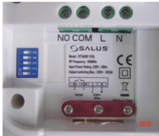
The wiring terminals and RF Address Code setting DIP switches are located on the rear of the Receiver, as shown in this picture:
