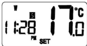
When any programme is running, the LCD display will show the programme set point temperature with the SET indicator displayed:
