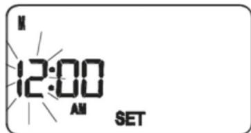
Press and hold SET and SELECT when the RT500RF is in Normal mode for a few seconds to enter the Clock setting mode. Release both keys and the display will look like the image below:
